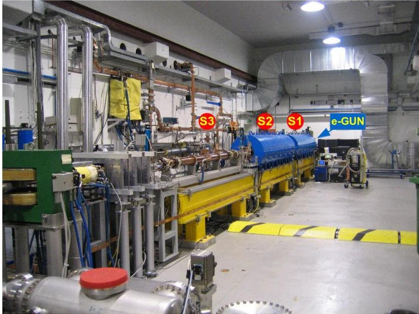
Figure 1.2: The SPARC\_LAB photo-injector. The electron gun, providing a  $5.6 \text{ MeV}$  beam energy, is followed by three TW accelerating sections (S1, S2 and S3), with the first two having solenoid coils embedded.
