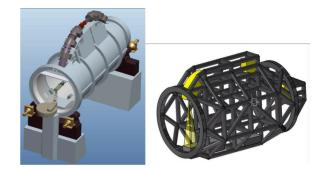
Figure 5: Design studies for iso-centric and superconducting carbon ion gantries. At NIRS/HIMAC (left) the planned 3T result in a radius of 5.5m whereas the concept presented by IBA/CEA (right) is based on 5.4T magnet design allowing for a very compact radius of 4m only.
