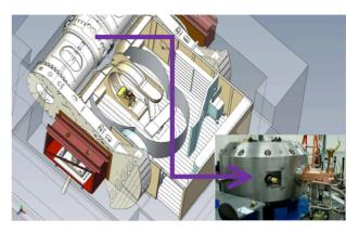
Figure 1: The Mevion S250<sup>®</sup> Proton Therapy System is based on a 9T, Nb3Sn, synchro-cyclotron that rotates closely around the patient.
