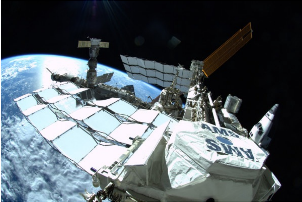
FIGURE 3.11 – Picture of the AMS-02 instrument place on its mission site on the ISS. Credits to Nasa.
