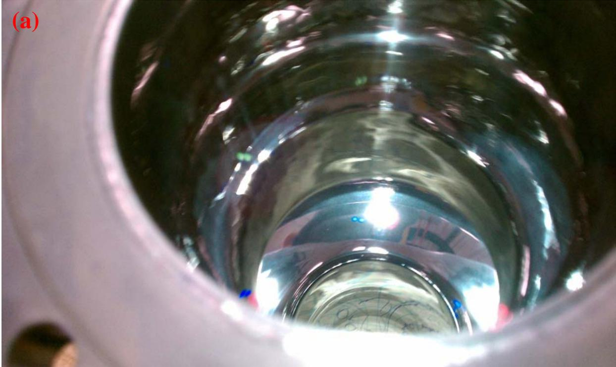
**Figure 2(a).** Pictures taken with a handheld digital camera of a single cell (a) and a nine cell (b) 1.3 GHz Tesla-type cavity after centrifugal barrel polishing to a mirror finish. The single cell cavity is standing on end on a piece of graph paper and the curved reflection of the grid can be seen in the cavity.
