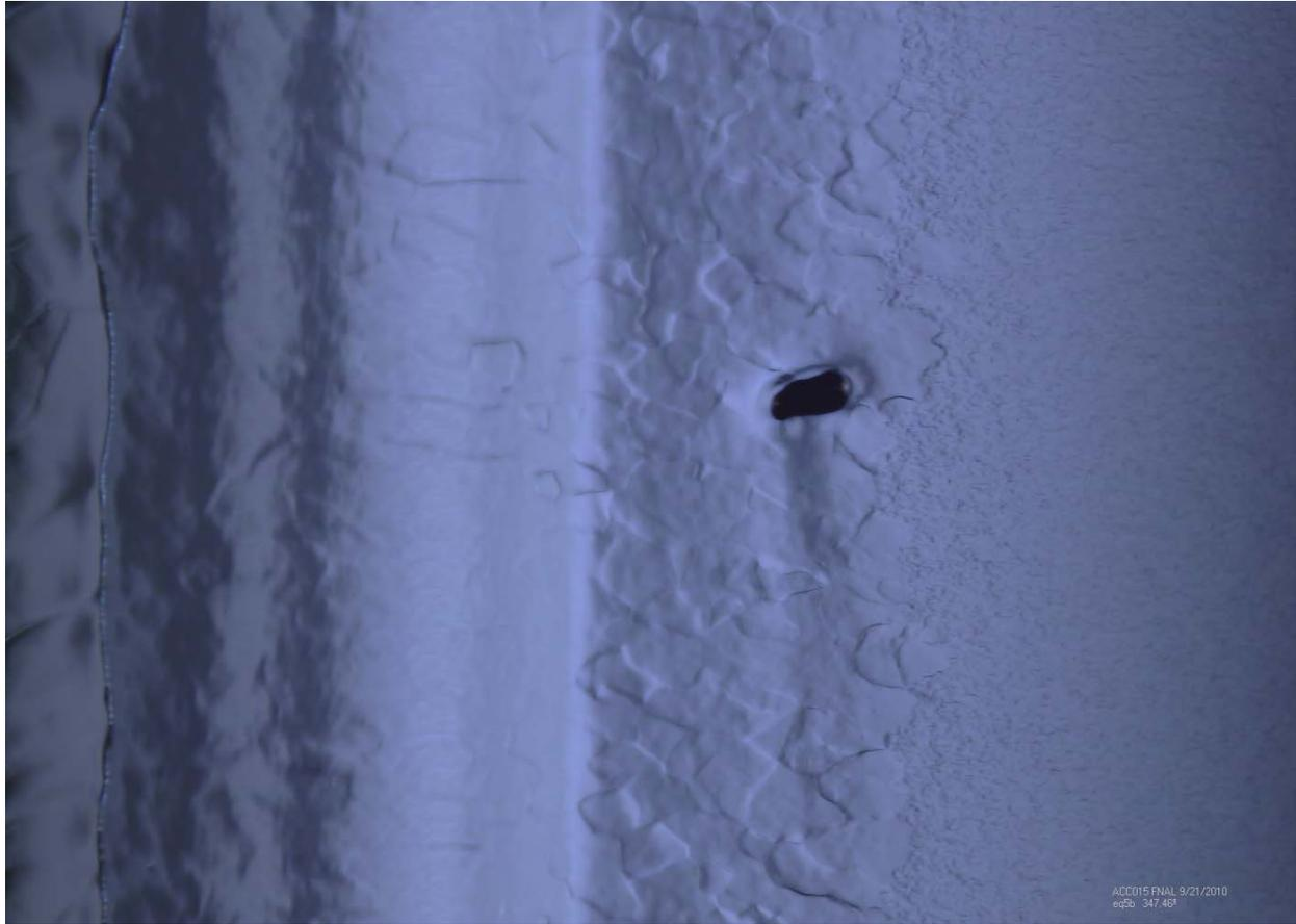
**Figure 7(a) shows a picture of the weld area of cavity TB9ACC015. There appears to be a large inclusion that was not removed by the standard electropolishing process.**
