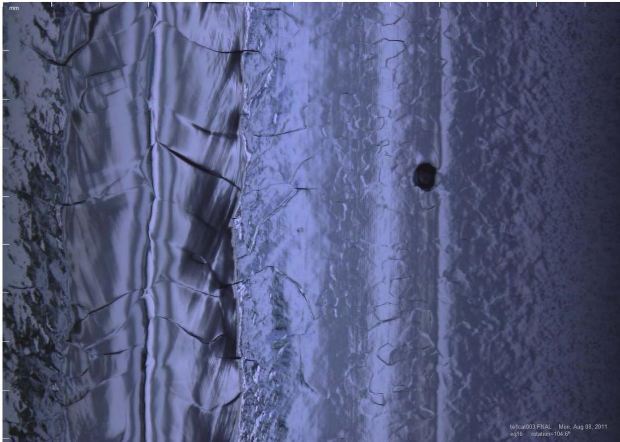
**Figure 5(b) shows the cavity at the same spot after the baseline electropolishing technique.**
