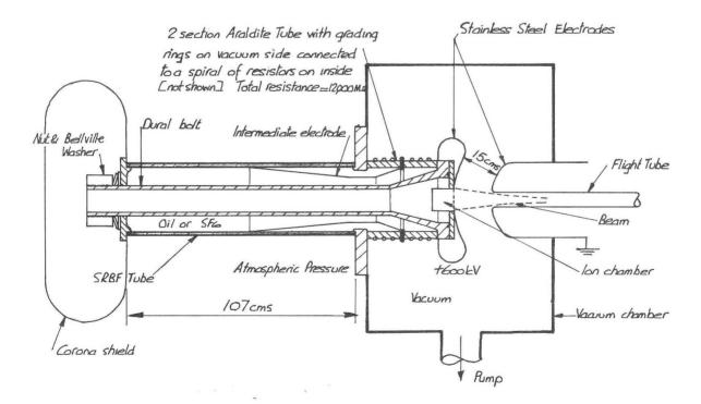
Fig. 2 Scaled-up lon Source with 600 kV Lead-in Bushing
