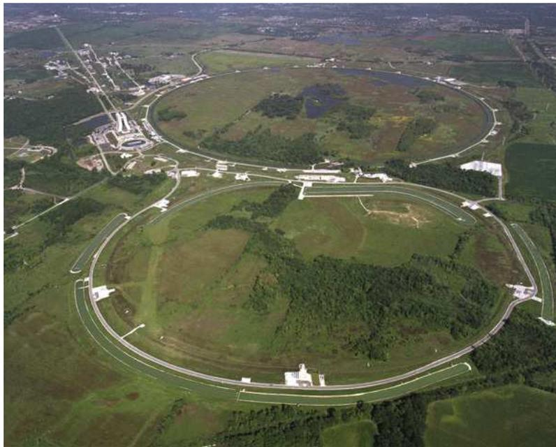
Figure 2.1: Aerial view of the Fermilab facility. The course of the Tevatron ring is indicated by the rear circular maintenance road.
