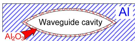
Figure 2: Cross-section of FEL waveguide.
