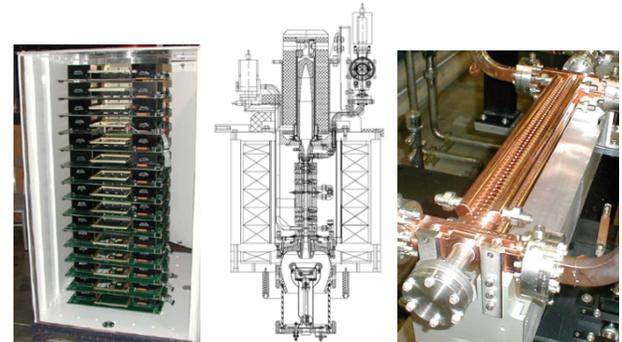
**Figure 4:** Solid state 400 kV modulator, SLAC XL4 50 MW 1.5  $\mu\text{s}$  X-band klystron, and a T53 X-band accelerator structure.
