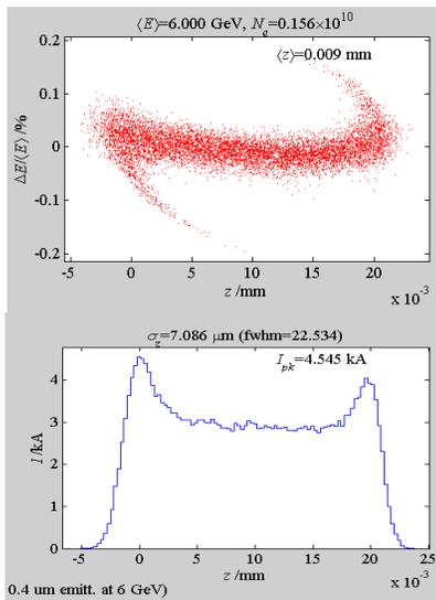
**Figure 2:** Litrack simulation results for longitudinal phase space and current profile after Linac-3 showing  $\sim 3$  kA peak current in the bunch core and almost no energy-z correlation (bunch head is at  $z < 0$ ).
