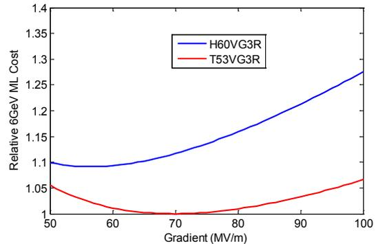
**Figure 6:** Dependence of the X-band 6 GeV main linac cost on acceleration gradient for the two structure types, normalized to the minimum for T53.
