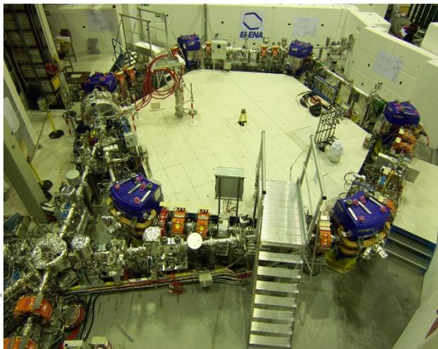
Figure 3: Installed ELENA ring with injection/ejection lines at bottom left and GBAR ejection line at top right.
