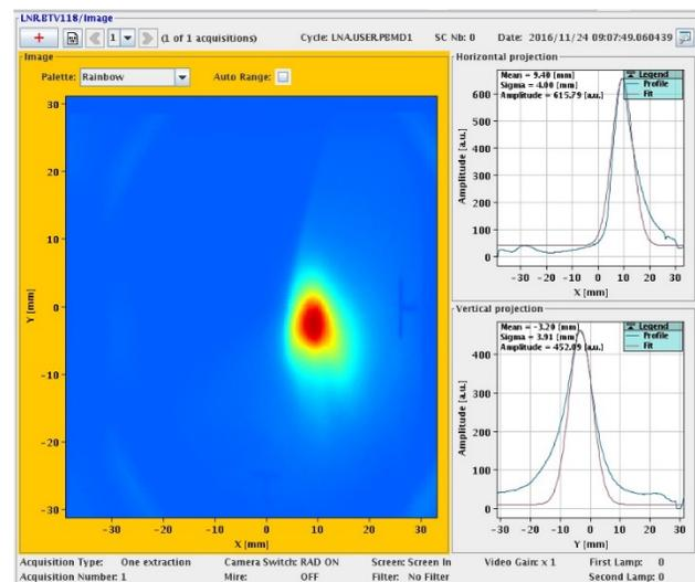
Figure 4: H<sup>-</sup> beam profiles as seen on BTV118.
