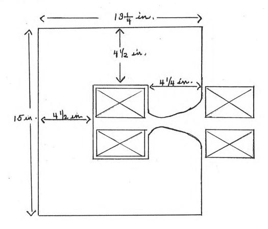
This leads to a coil cross-section about 4 inches by 2-1/4 inches. Scaled from the A.G.S. the magnet's minimum gap is just a little over 3/4 inch and the pole tip width is about 4-1/4 inch. Other magnet dimensions might be as shown in the figure. Approximate weights are, then, about 6000 tons of steel and about 1400 tons of copper. Thus the estimates are:
