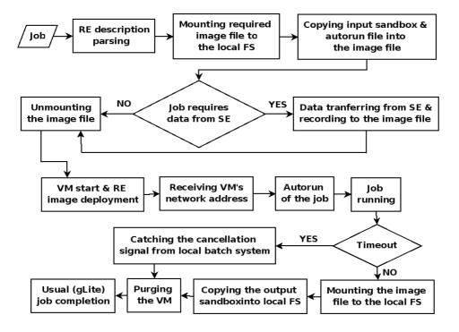
Fig. 1. Algorithm of job processing by a modified WN
