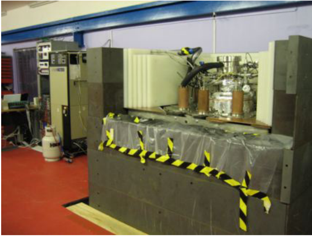
Figure 2. The ZEPLIN II detector running underground. The lead shielding and moderator have been partially removed. The target is surrounded by an organic liquid scintillator veto read out by 10 photomultiplier tubes, 3 of whose housings are visible in the foreground. The outer vacuum jacket is made of stainless steel, the inner pressure vessel housing the xenon is made of copper. All electrical and gas connections are to a manifold on top of the target volume. The black insulated line connected to this manifold is the return line for the refrigerant. The target is maintained at 163K by a commercial refrigerator, visible immediately behind the edge of the shielding. The rack behind the refrigerator contains the slow control and trigger electronics. The events are digitized in a 2ns sampling Acqiris ADC visible on the table in the background.
