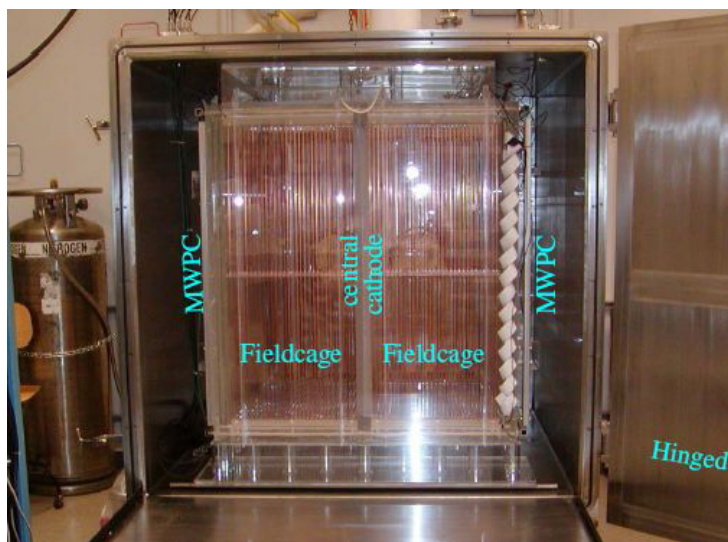
Figure 5. The first DRIFT II module during test assembly. The completed detector is now taking production data underground at Boulby.
