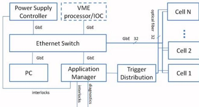
**Figure 2.** Controls block diagram for the P2 Marx modulator. Presently, a PC is used to control the modulator state, and view and store diagnostics. A planned upgrade is to migrate this functionality to a VME/EPICs based system.
