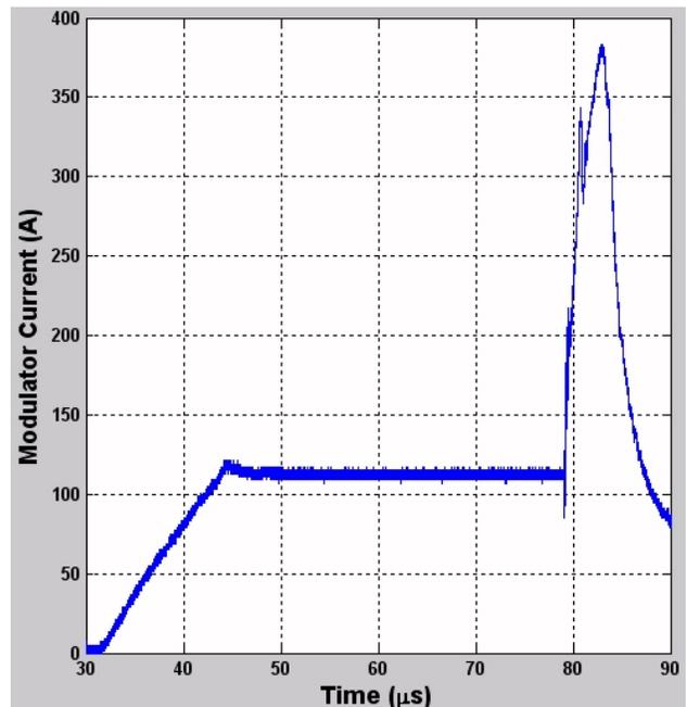
Figure 7. Measured modulator current before and during an arc. At  $\sim 78 \mu$ s a self-break spark gap across the load closes. This test was performed at 120kV modulator output voltage.
