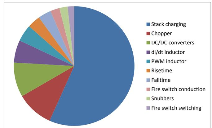
**Figure 4.** Calculated distribution of losses for a typical P2 Marx cell.
