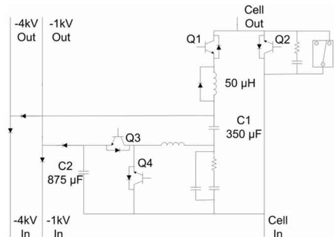
Figure 1. P2 Marx single-cell simplified circuit schematic.
