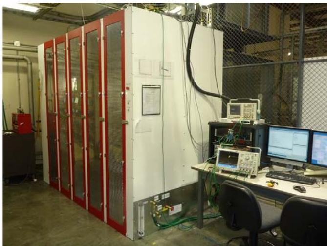
**Figure 3.** Photograph of the P2 Marx modulator.
