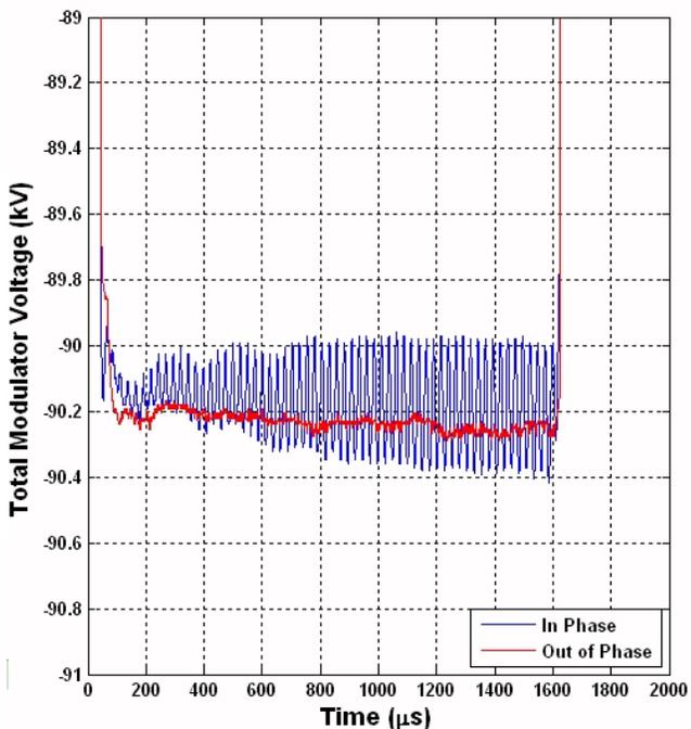
Figure 6. Measured output voltage of the modulator operating into a water load. Flat-top portion of cell is highlighted. The blue trace shows when the cell PWM timings are synchronized “in-phase” and the red trace shows when they are placed out of phase.
