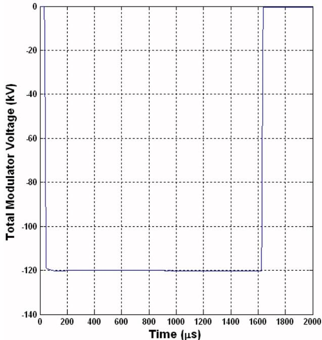
Figure 5. Measured modulator output voltage into a water load.
