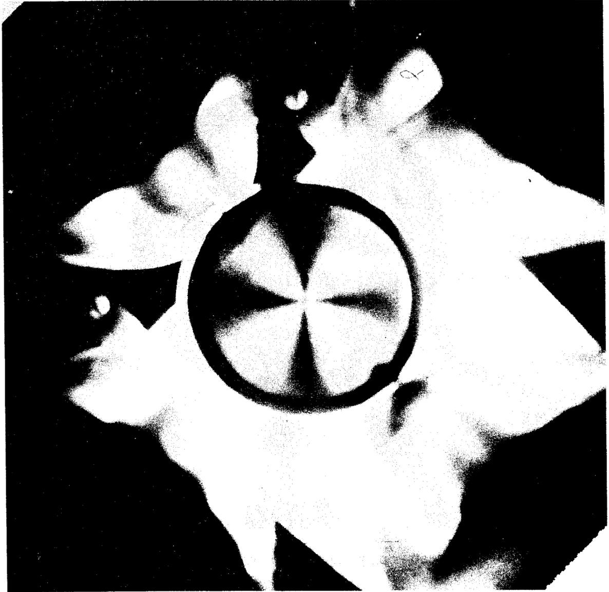
Fig. 2--Light scattering pattern in a quadrupole magnetic field ( $\phi = 0$ ).
