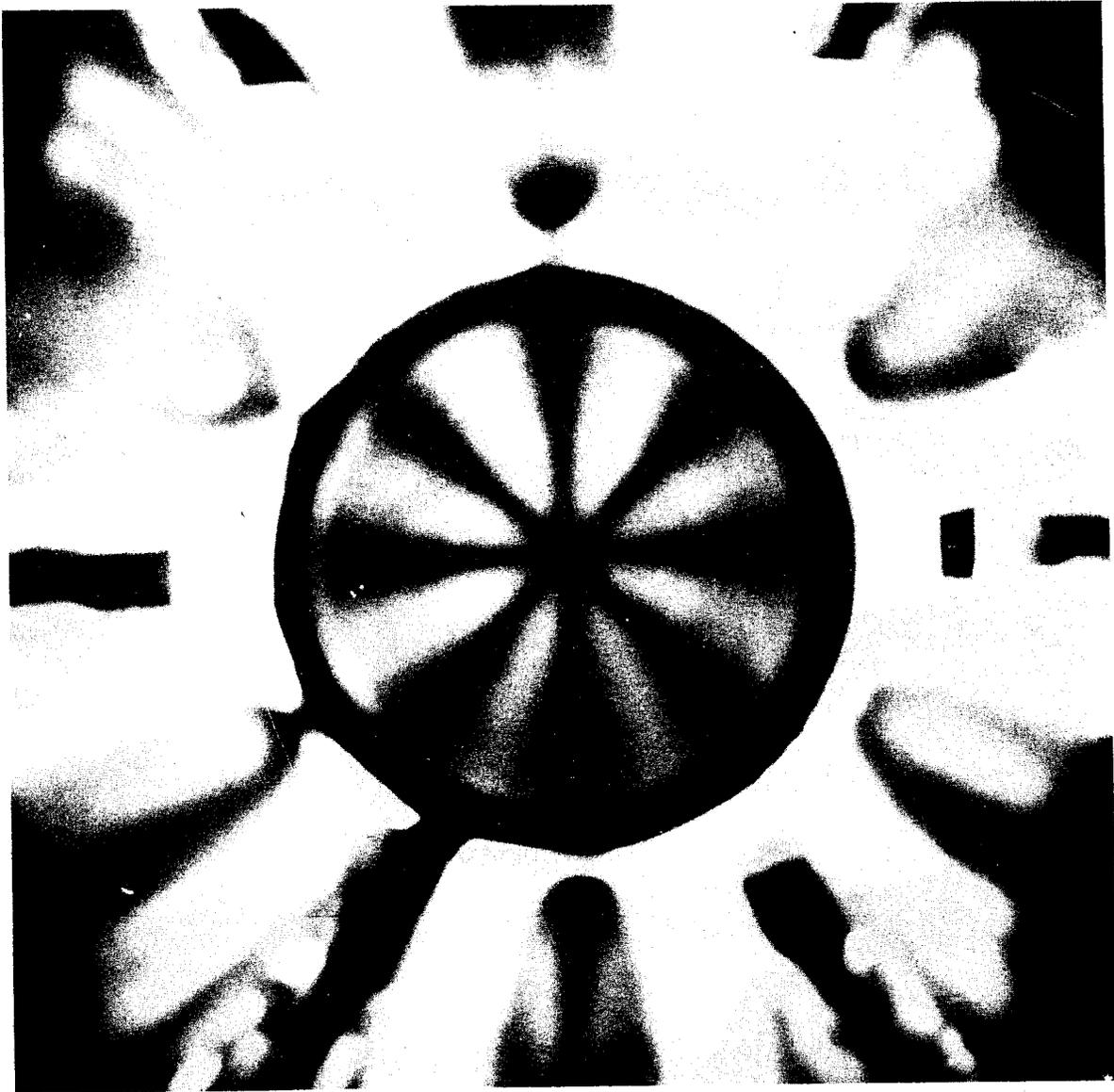
Fig. 3--Light scattering pattern in a sextupole magnetic field ( $\phi = 0$ ).
