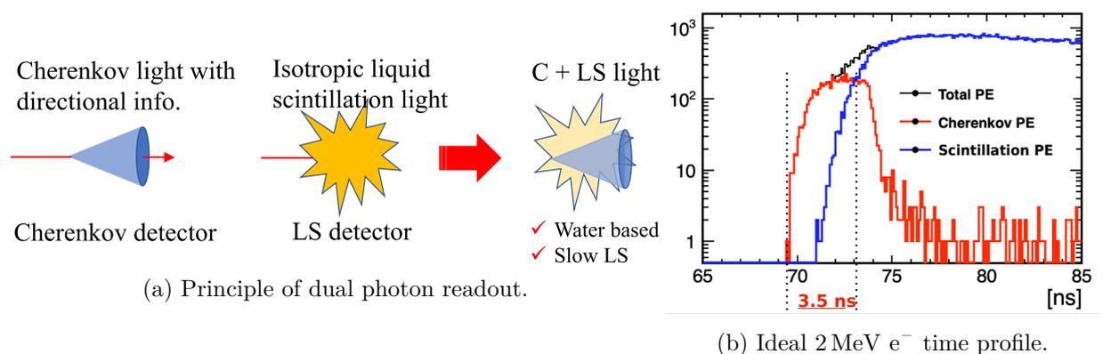
Figure 2: Cherenkov scintillation dual photon readout. Under ideal assumptions, 2 MeV electron can give a 3.5 ns Cherenkov time window.
