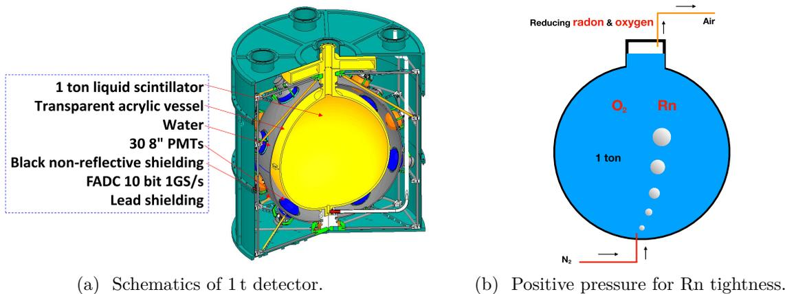
Figure 1: 1 t prototype detector for background measurement, purification development, and slow liquid scintillator performance assessment.
