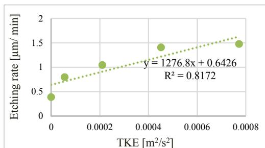
Figure 4: Measured etching rate as a function of the simulated TKE.
