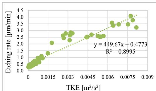
Figure 9: Correlation etching rate from mock-up test vs TKE.
