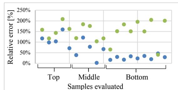
Figure 6: Relative error from: ● Correlation etching rate-shear rate ● Correlation etching rate TKE.
