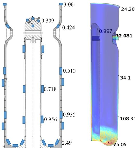
Figure 7: Local etching rates [ $\mu\text{m}/\text{min}$ ] from the mock-up cavity and calculation of the shear rate [ $\text{s}^{-1}$ ] in this locations.
