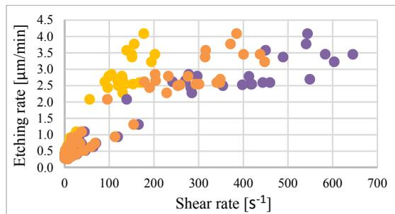
Figure 11: Comparison correlation etching rate-shear rate obtained with different meshes: ● Initial mesh ● 2<sup>nd</sup> mesh (13 layers) ● 3<sup>rd</sup> mesh (16 layers).
