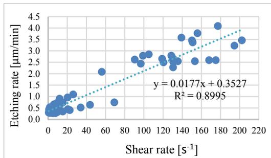
Figure 8: Correlation etching rate from mock-up test vs shear rate.
