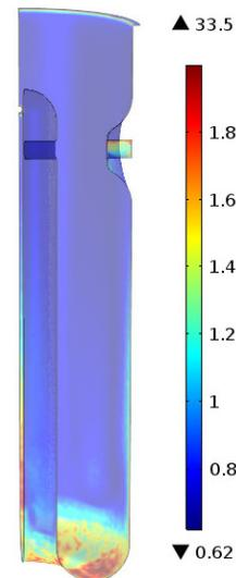
Figure 5: Etching rate distribution [ $\mu\text{m}/\text{min}$ ] in HIE-ISOLDE obtained using the correlation in Fig. 3.
