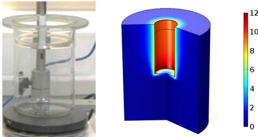
Figure 2: Laboratory set-up; Shear rate distribution [ $\text{s}^{-1}$ ] resulting from the simulation.
