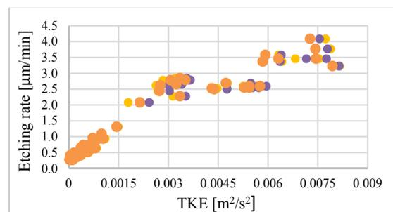
Figure 12: Comparison correlation etching rate-TKE obtained with different meshes: ● Initial mesh ● 2<sup>nd</sup> mesh (13 layers) ● 3<sup>rd</sup> mesh (16 layers).
