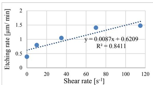
Figure 3: Measured etching rate as a function of the simulated shear rate.
