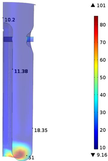
Figure 14. Distribution of the thickness removed [ $\mu\text{m}$ ] in the chemical polishing.
