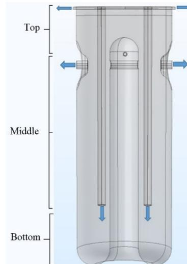
Figure 1: Scheme with the SUBU bath inlets and outlets during the polishing process.
