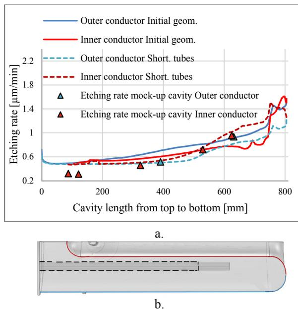
Figure 13: a. Comparison between the etching rate of the inner and outer conductor using different tube lengths; b. Cavity cross section with inner and outer conductor.
