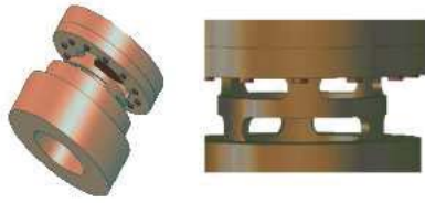
Figure 1. Scheme of the 5th transducer generation. The lower ring (left) is introduced in the sphere holes. The middle part works as a spring, which will be tuned to the sphere resonant frequency at low temperature. The upper part contains the electromagnetic resonant cavity, which is closed by a 50\ \mu\text{m} membrane thick. This transducer is \sim 30\ \text{mm} diameter [7].
