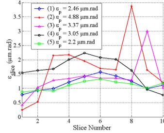
Figure 5. Slice emittance from PARMELA with different distribution for the 1.5 mm diameter emission spot and  $I_{sol} = 104$  A; (1) uniform disk, (2) high emission region  $r=0.15$ mm, 10% out of 10k particles, (3) same as (2) with 5%, (4) hole of  $r = 0.15$  mm in uniform disk, (5) same as (1) but  $I_{sol} = 116$  A
