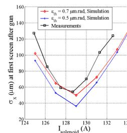
Figure 1. Beam spot sizes vs solenoid current,  $r_{spot} = 0.75$  mm; the simulated curve with a thermal emittance of 0.5 mm.mrad has the curvature of the measured one
