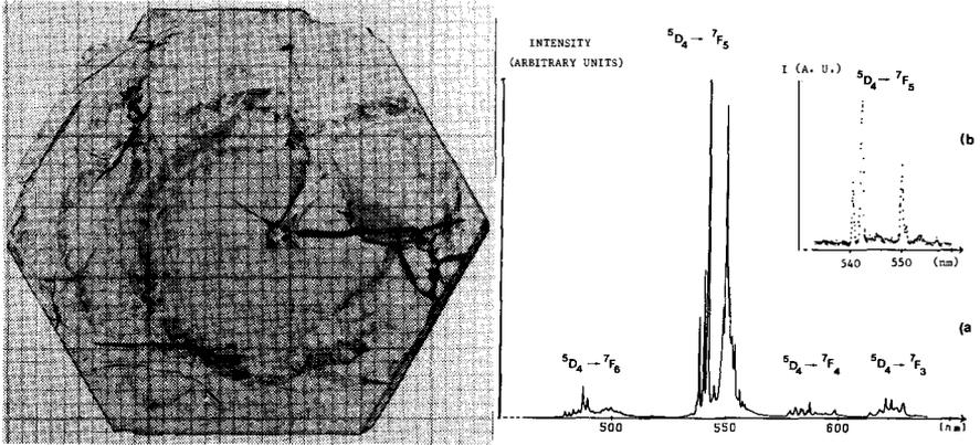
Fig. 1 (left) - Transparent single  $InBO_3$  crystal grown by the flux method.
