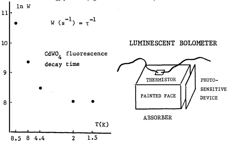
Fig. 4 (left) - Fluorescence decay time of  $CdWO_4$  at 500 nm emission wavelength and 2935 Å excitation wavelength, in terms of temperature between 8.5 K and 1.5 K .
