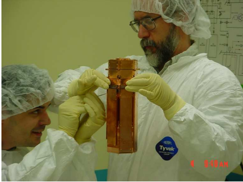
Figure 3.12: Dan Bauer (right) and Vuk Mandic (left) look at one of the towers. The 6 detectors in the tower are in the 1.2 cm tall copper houses at the bottom of the copper structure. The long, vertical, copper extender cards carry signals between the detectors and the cold electronics which are mounted like a crown on top.
