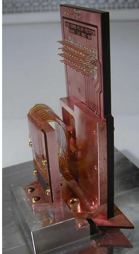
Figure 3.18: A picture of a SQUET card. A SQUET card is used to amplify the ionization and phonon signals from a detector. The ionization signals are amplified by field effect transistors (FETs) which are located in the enclosed copper area. The FETs operate at 4 K. The phonon signals are amplified by the arrays of SQUIDS. The SQUID arrays are located on the smaller part of the card to the left and operate at 600 mK. A SQUET card is mounted to the top of a tower of detectors. A stripline, which connects to the pins at the top of the card, carries the ionization and phonon signals out to the detector electronics.
