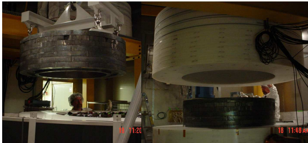
Figure 3.11: A view of the top of the lead and poly shield as they are being lowered into place. On the left, Dave Hale guides the lead lid into place. On the right, Dave Hale motions the poly lid into place.
