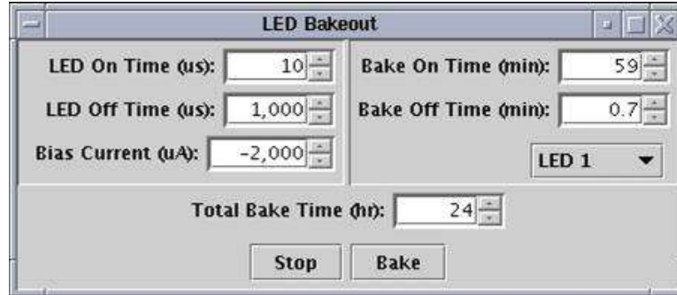
Figure 3.30: A picture of the bake GUI. The bake GUI allows the user to specify the LED flashing parameters used to neutralize the detectors.
