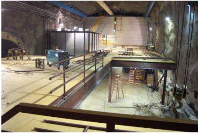
Figure 3.3: A view of CDMS in the Soudan Underground Laboratory. The picture is taken on top of the mezzanine looking south. To the left, the top of the RF-shielded clean room housing the detectors can be seen protruding through the mezzanine. Immediately behind the clean room is the DAQ room. Through the tunnel, the top of which can be seen to the far left, is the chamber housing the MINOS experiment. Behind the white wall is where the Soudan2 experiment was located before it was removed. After this picture was taken, a ping pong table, which was particularly useful for sanity preservation, was located on the far right hand side of the mezzanine.
