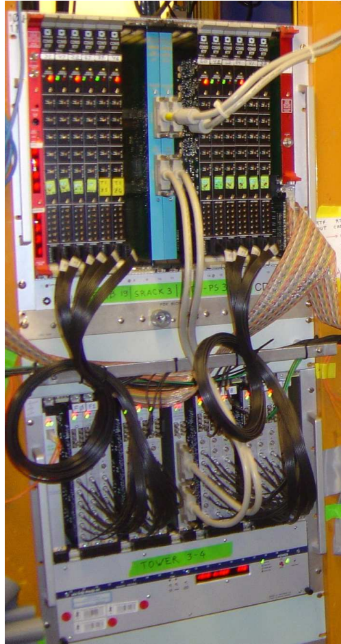
Figure 3.21: A picture of the RTF crate (upper) containing the RTF boards and TCBs and the VME crate (lower) containing the digitizers and history buffer. The 2 blue cards in the center of the upper crate are the TCBs. The 6 black cards to the left of the TCBs and the 6 black cards to the right of the TCBs are the RTF boards. Black ribbon cables carry the phonon and ionization pulses from the RTF boards to the digitizers in the VME crate. The lower (upper) SCSI cables from the TCBs head to the history buffer in the VME crate (head to the TLB which is not shown). The left-most card in the VME crate is the VME-to-PCI bridge.
