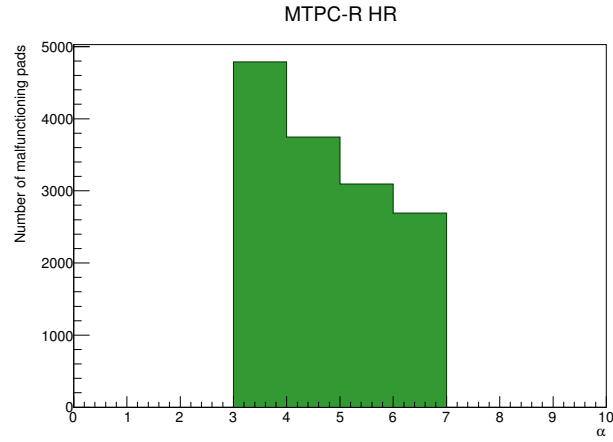
FIGURE 4.23: Plot of the integral parameter \alpha value and number of malfunctioning pads found. From this plot we estimate \alpha = 4
