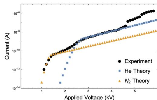
**Figure 6.** Fit of theoretical nitrogen and helium I-V curves to data.
