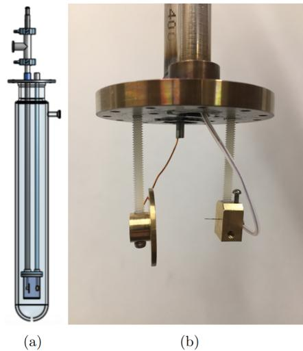
**Figure 4.** (a) The experimental can suspended in a glass dewar and (b) the brass cathode and tungsten nanotip suspended from the roof of the can by threaded nylon rods.
