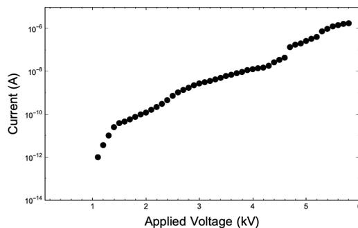
**Figure 5.** I-V curve for air mixed with helium at room temp. and 1 atm.
