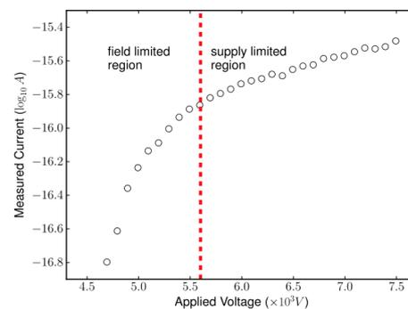
**Figure 3.** Field ionization data of He from a W tip taken by O'Donnell [5]. The field limited and supply limited regions are highlighted.
