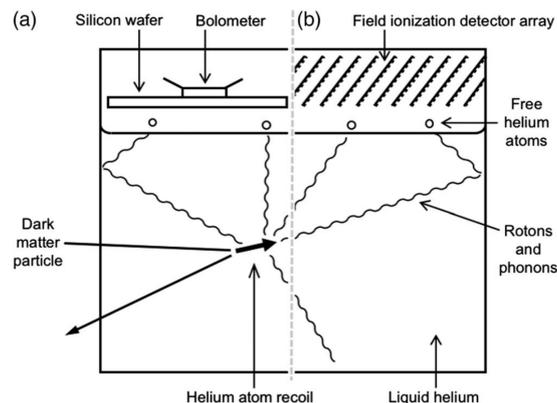
**Figure 1.** Schematic diagram of (a) The HERON detector and (b) the proposed detector. In both cases the collision between a dark matter particle and a helium nucleus results in phonons and rotons which, upon arriving at the surface, eject helium atoms by quantum evaporation. [4]
