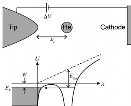
**Figure 2.** Illustration of a He atom near a positively charged metal tip and the potential energy  $U$  seen by the bound electron. [4]
