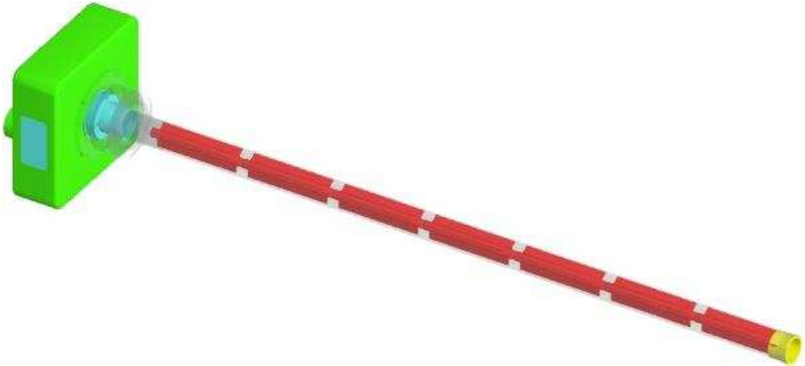
Figure 3.2: A engineering diagram of the BNB beryllium target. The proton beam enters from the left.
