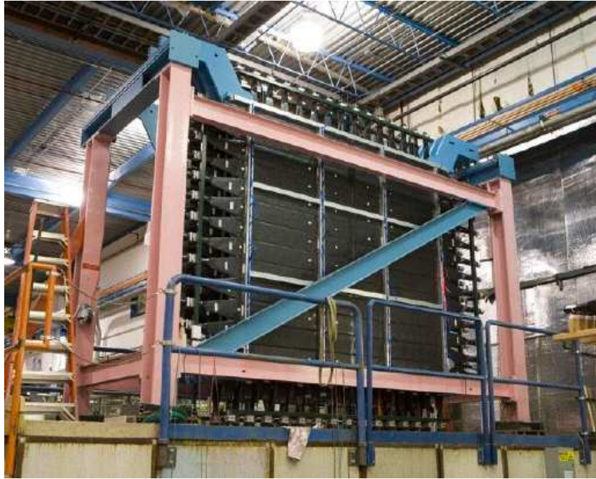
Figure 3.6: The MRD at the assembly point in Lab F of Fermilab. Black, light tight, scintillator counters are arranged in pairs in alternating horizontal and vertical planes, and are strapped to a (silver) aluminum frame with (blue) nylon. The PMTs are read out on the top, bottom and sides of detector. The (blue) iron planes sit on a (pink) support frame.
