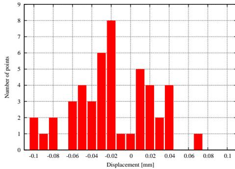
Figure 6: Histogram of displacements of quadrupole magnets
