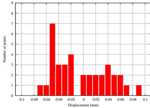
Figure 5: Histogram of displacements of bending magnets
