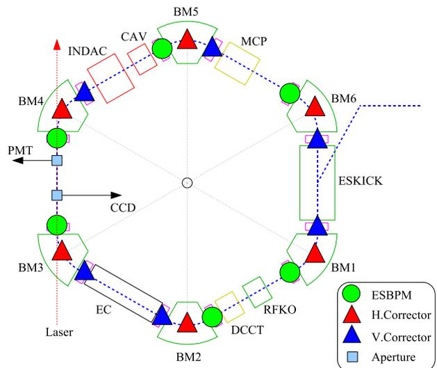
Figure 7: Device layout of COD correction
