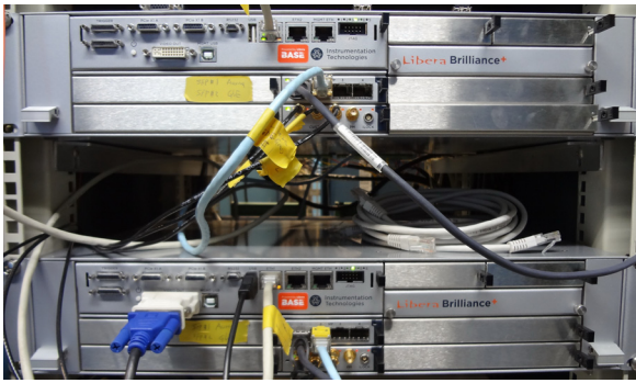
Figure 3: Feedback system platform.
