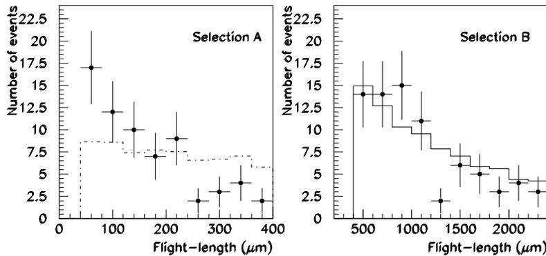
Figure 3: Flight-length distributions of charged charm candidates decaying into three particles. The histograms represent the flight-length distributions given by the Monte Carlo simulation for  $D^+$  and  $D_s^+$ , normalized to the number of observed events.
