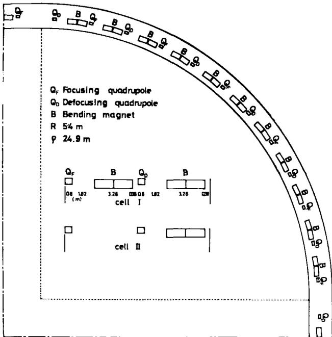
Fig.14 Cell Structure of KEK Main Ring
