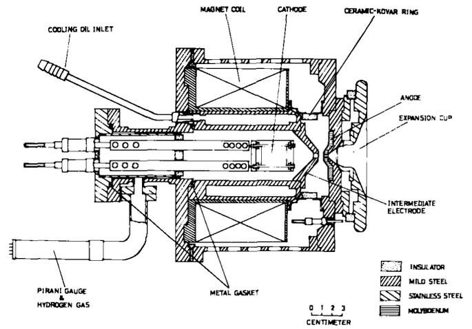
Fig.4 Duoplasmatron with a Nozzle-type Expansion Cup
