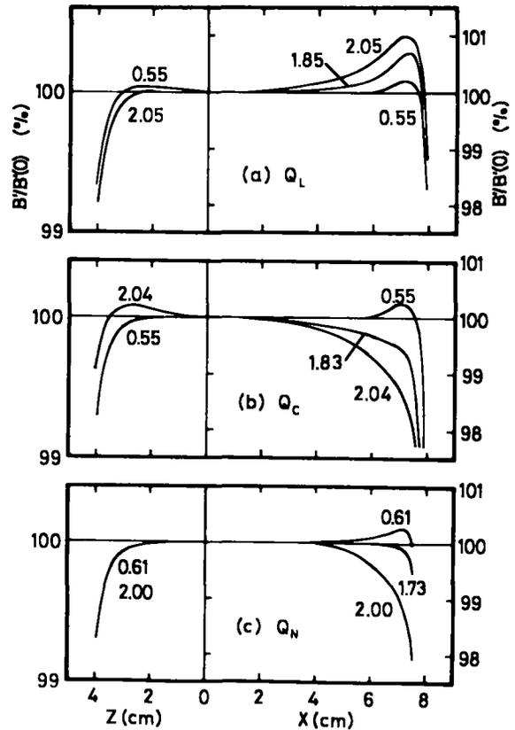
Fig.16 Horizontal and Vertical Gradient Distributions of Quadrupole Magnet. See ref.11.
