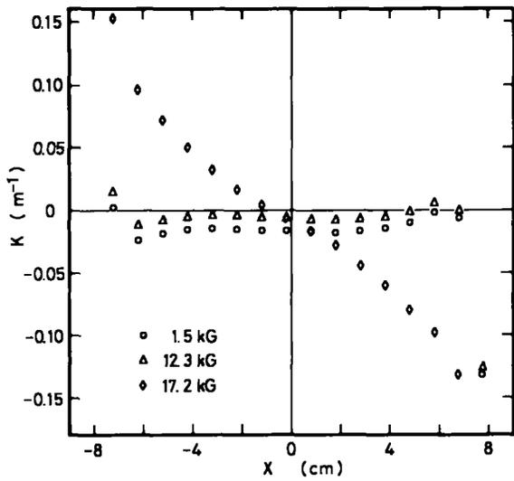
Fig.18 Gradient Distribution of Bending Magnet
