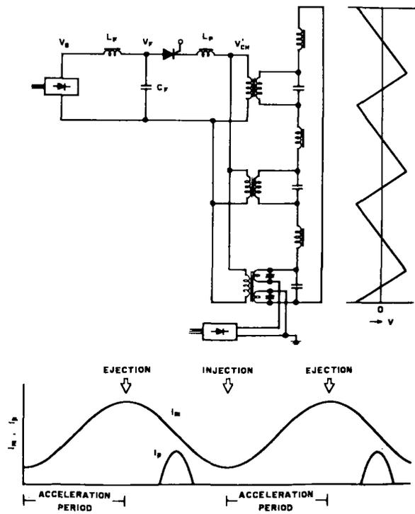
Fig.10 Basic Diagram of Booster Power Circuit
