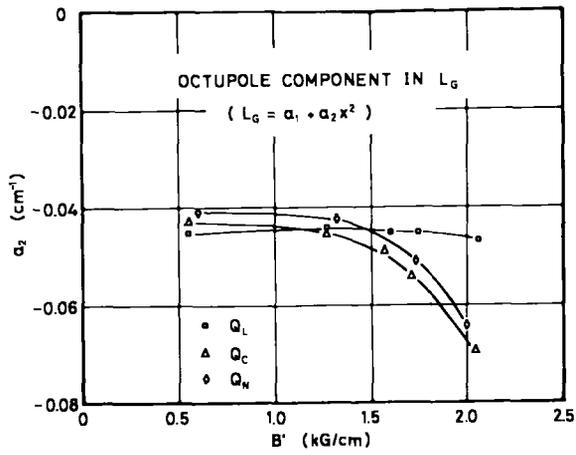
Fig.17 Octupole Component of Effective Length of Quadrupole Magnet
