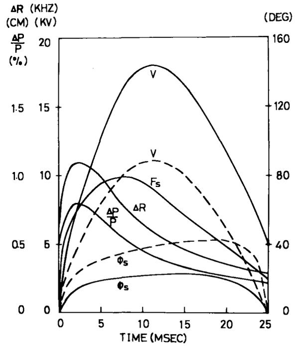
Fig.13 RF Program of Booster. Broken Curves show Necessary Minimum Voltage and Corresponding Phase Stable Angle.  $F_s$  gives Frequency of Phase Oscillations.
