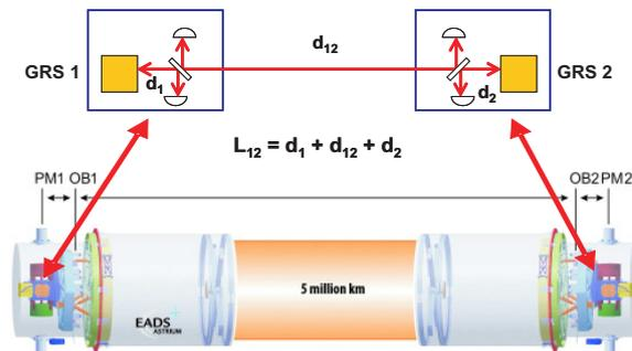
**Figure 1.** Schematic of the strap-down-architecture. The distance measurement is split into two local, from proof mass (PM) to the optical bench (OB), and one long distance measurement.
