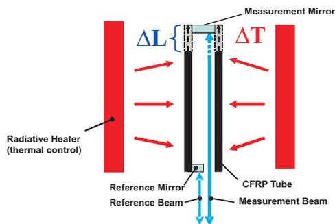
**Figure 7.** Sketch of our CTE measurement facility.
