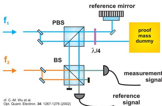
**Figure 2.** Schematic of the heterodyne interferometer (BS: beamsplitter; PBS: polarizing beamsplitter). The signal at the photodiodes are given by  $I_{meas} \sim AB \cdot \cos(\Delta\omega t - \phi(t))$  and  $I_{ref} \sim AB \cdot \cos(\Delta\omega t)$ . Here, A and B denote the amplitudes of the laser,  $f_1$  and  $f_2$  the frequencies and  $\Delta\omega = 2\pi|f_1 - f_2|$ .
