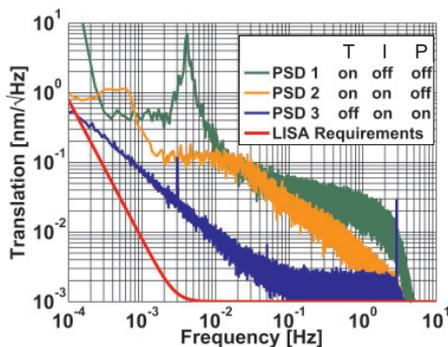
**Figure 5.** Power spectrum densities (PSD) of the translation noise measurements. The smooth line at the bottom represents the LISA requirements. At the beginning (upper line) with temperature stabilization (T) but without intensity- (I) and phase- (P) stabilization. The lower line represents the current noise performance.
