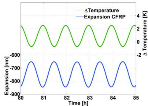
**Figure 8.** Typical time series of a CTE measurement run. The upper curve represents the cycled temperature of the CFRP probe, the lower curve the measured expansion.
