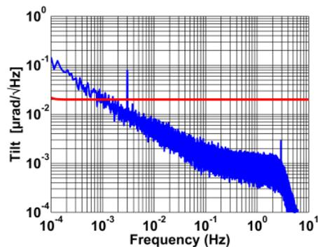
**Figure 6.** PSD of the tilt noise measurement (T: off, I: on, P: on). The smooth line represents the DFACS requirements. The roll off at 3 Hz is caused by a digital low pass filter in the data acquisition chain.
