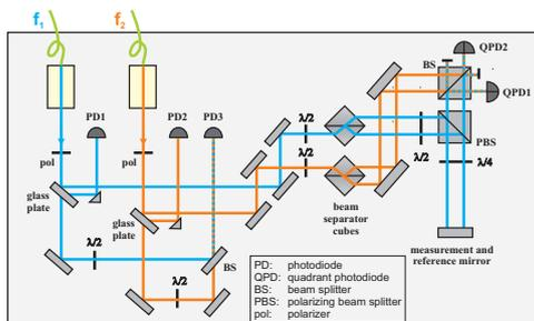
**Figure 3.** Schematic of the heterodyne interferometer.
