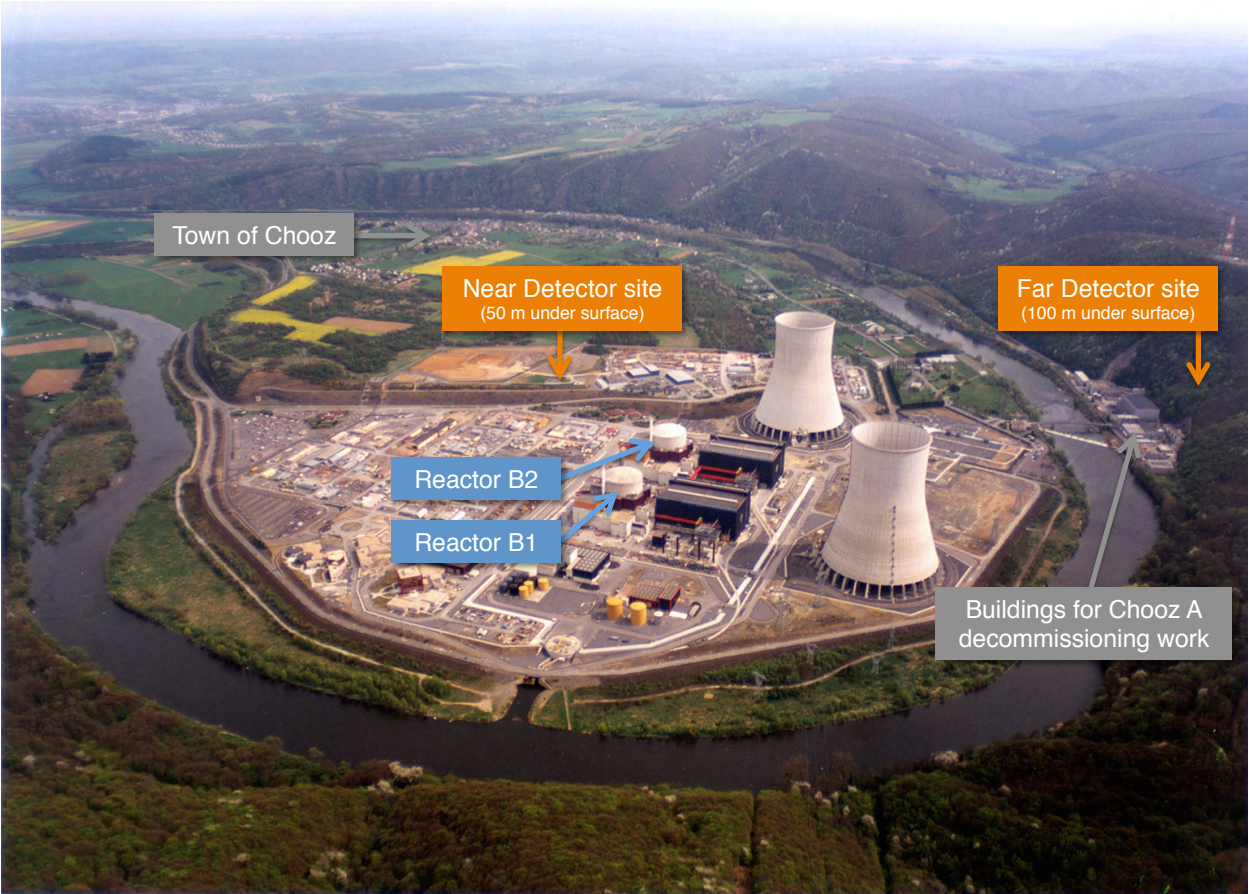
Figure 7.1: The site of the Double Chooz experiment, highlighting the two operating reactors, B1 and B2; buildings used for decommissioning of the Chooz A reactor; and the locations of the two Double Chooz detectors (both underground, as indicated in the labels). The town of Chooz is also identified.
